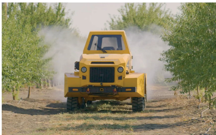
Bonsai Robotics has designed a vision-based technology that allows farm vehicles to autonomously traverse orchards faster than machinery operated by people. Photo: Bonsai Robotics
